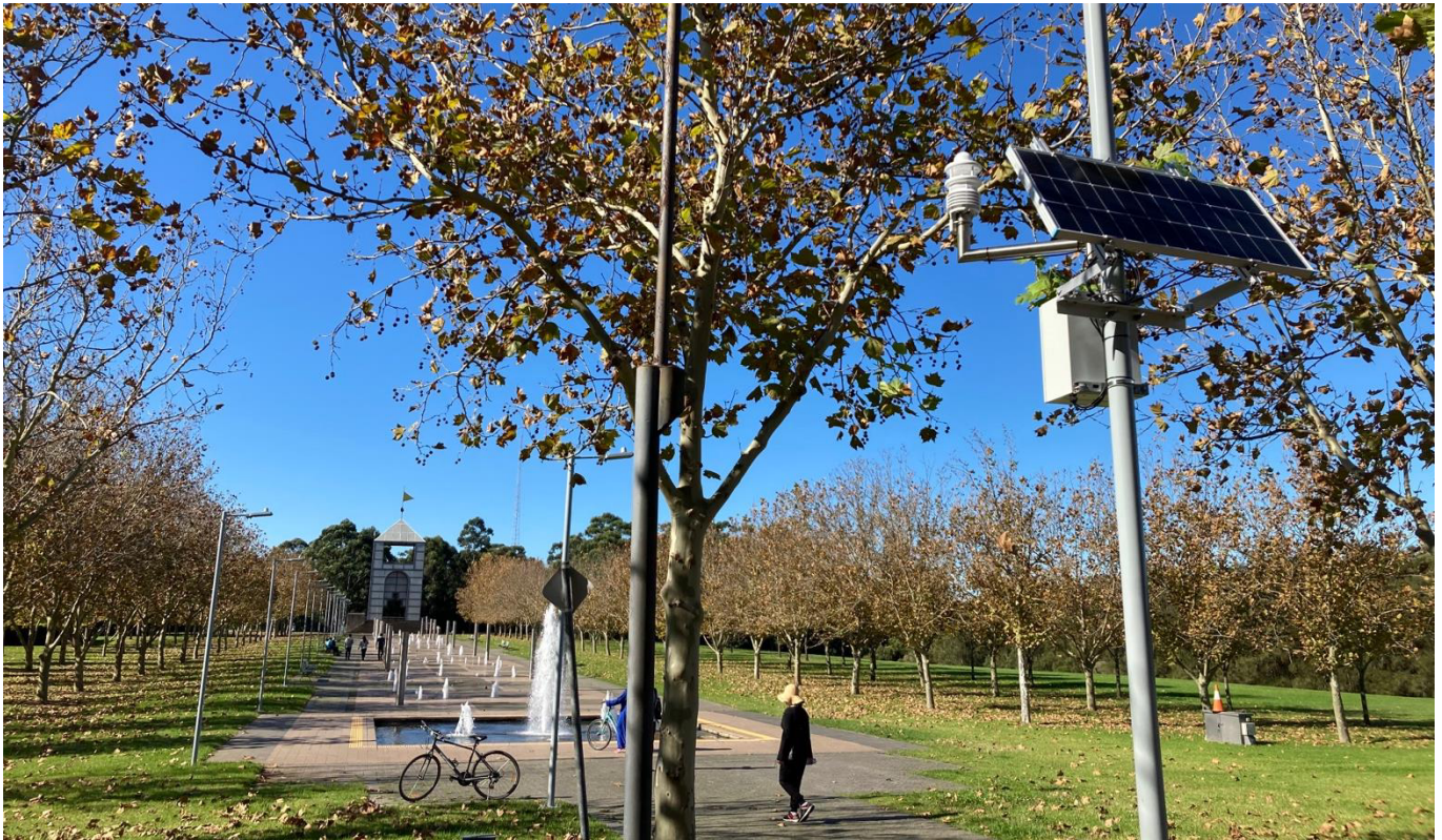
A weather station at Sydney Olympic Park provides a range of secondary meteorological data to support the interpretation of urban heat data from a network of 50 low-cost temperature and humidity sensors. Image source: UTS
