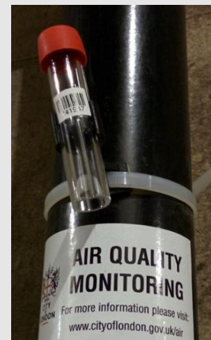
A gas diffusion tube used by the City of London. Image source: Creative Commons
