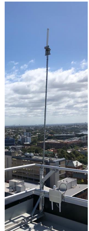
A LoRaWAN gateway on a rooftop in Sydney, Australia. Image source: UTS
