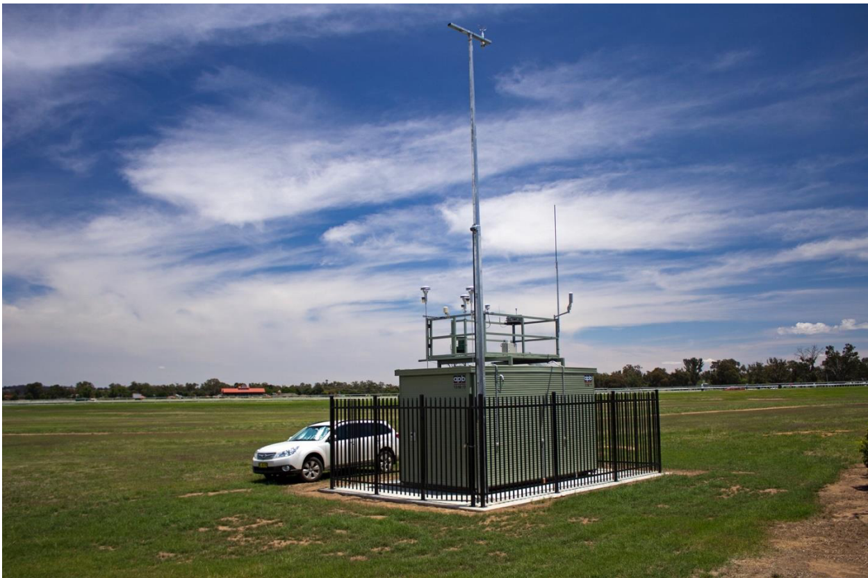
A regulatory ambient air quality monitoring station in Wagga Wagga (NSW) that is part of the NSW Government's state-wide monitoring network. Stations like this one produce high-quality reference data that can be used to verify data from low-cost sensors. Image source: Creative Commons
