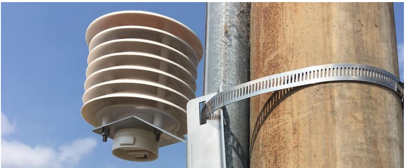
A Stevenson shield can protect sensors from thermal radiation and direct sun while maintaining optimal airflow. Image source: UTS.
