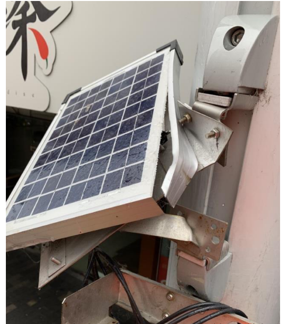
A sensing device solar panel damaged by collision with a delivery truck in the City of Sydney. Image source: UTS
