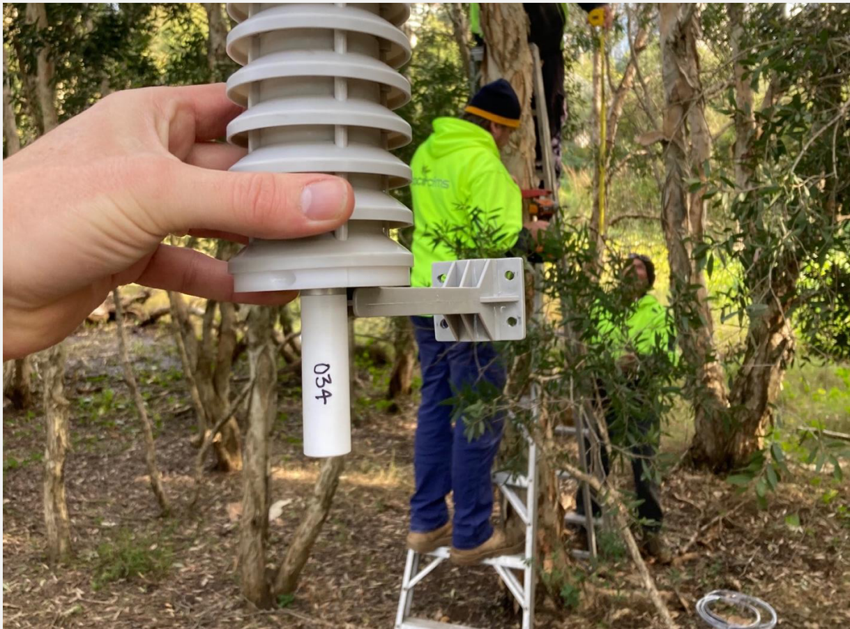
An example of a photograph that shows a device ID number relative to its deployment context. Image source: UTS
