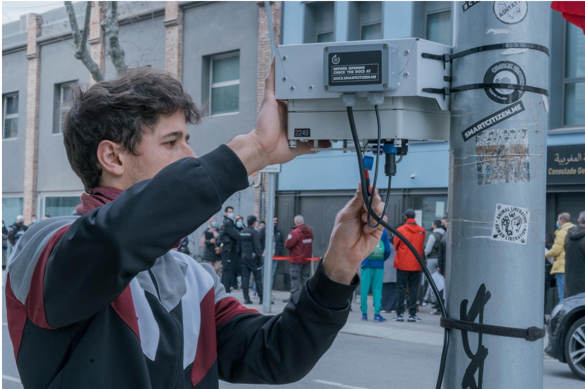
A community participant carries out maintenance on a Smart Citizen air quality sensing device in Barcelona, Spain. Image source: Creative Commons
