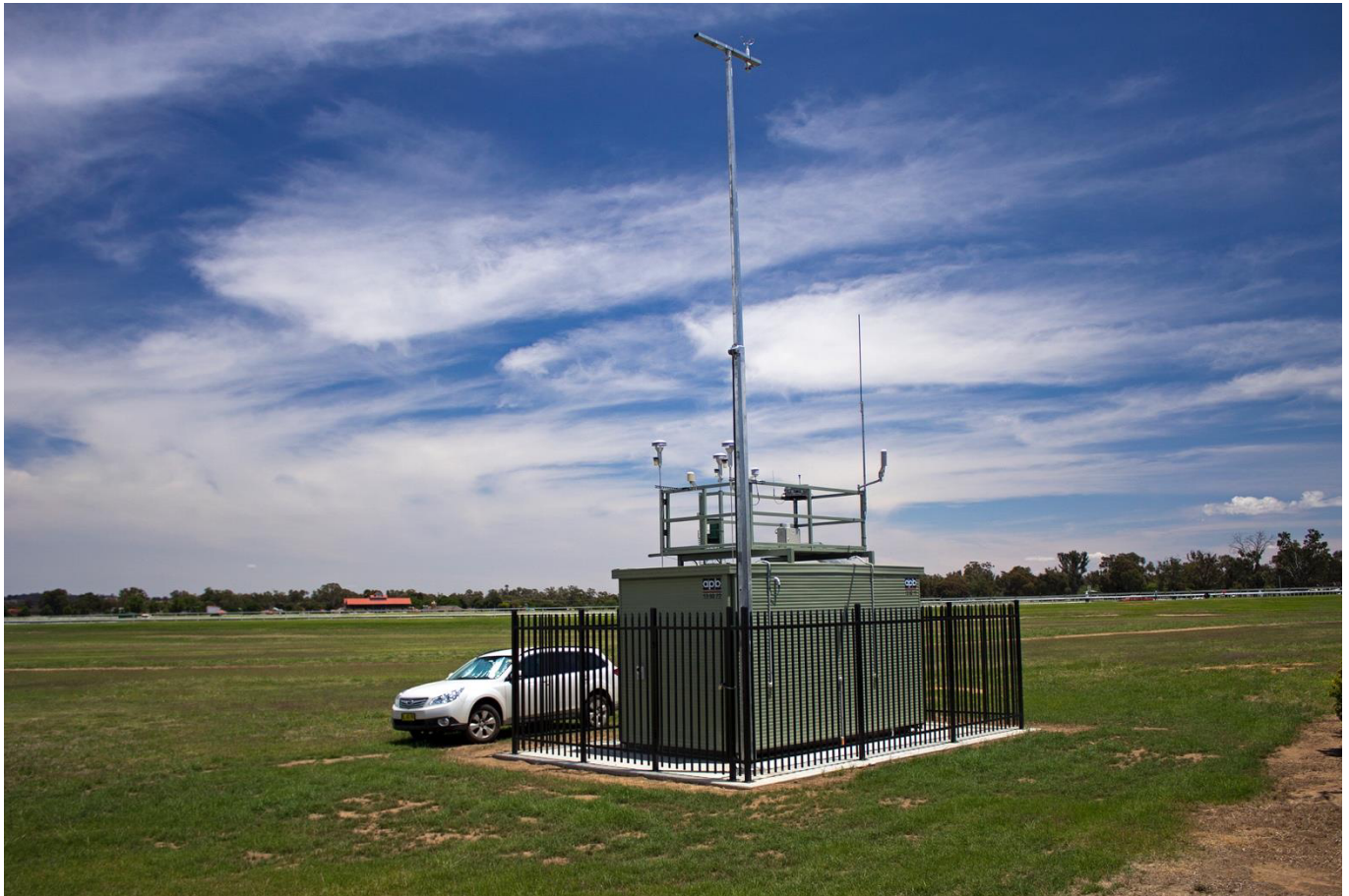
A regulatory ambient air quality monitoring station in Wagga Wagga (NSW), part of the NSW government's state-wide monitoring network. Image source: Creative Commons
